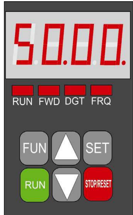
7-segment display, status LED and keypads
